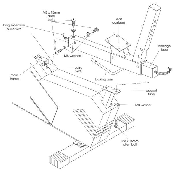
Figure 3 - Install Seat Carriage
